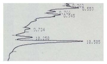
Figure 2: Chromatogram of cucumber sample with added azoxystrobin in concentration of 0.05 mg/kg
