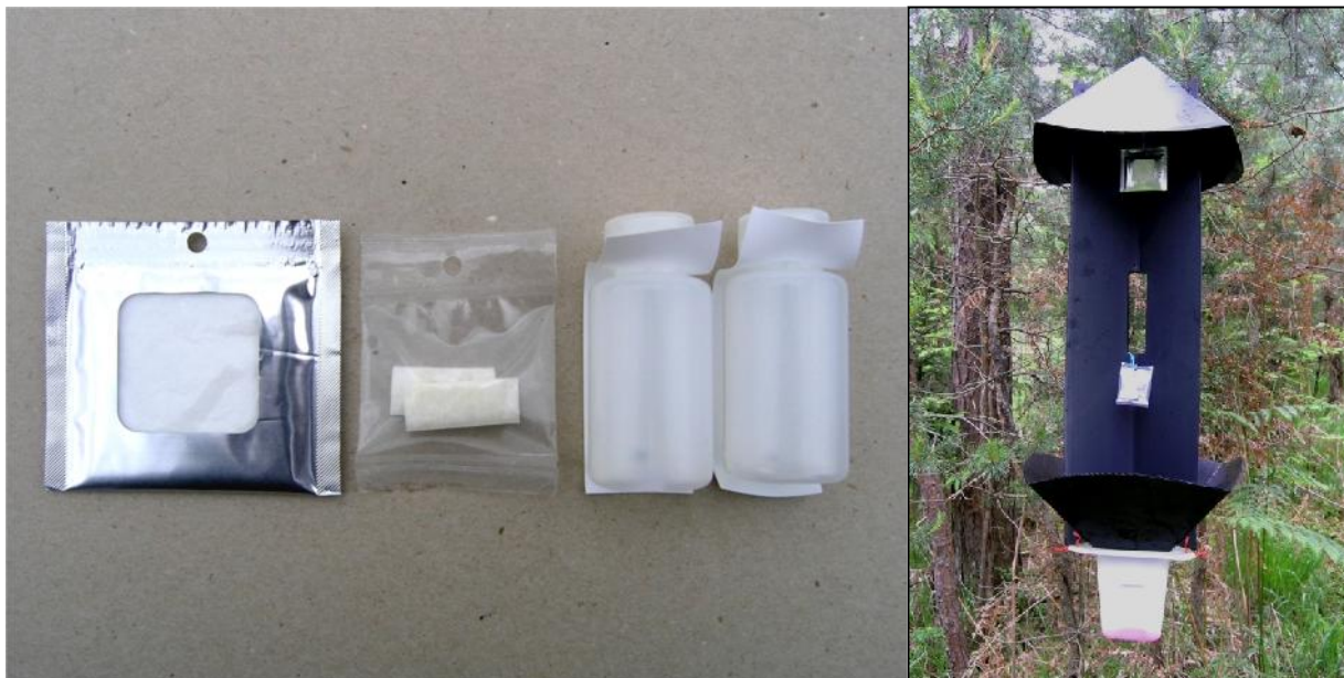
Slika 1: Sestavine atraktanta Galloprotect Pack ® - Galloprotect F, Galloprotect A in Galloprotect Plus (levo) in križna cevna past Witasek, opremljena z atraktantom Galloprotect 2D ® (desno) (foto: Roman Pavlin).
